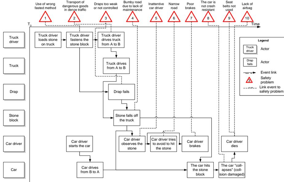
Figure 25. Step worksheet with safety problems.
