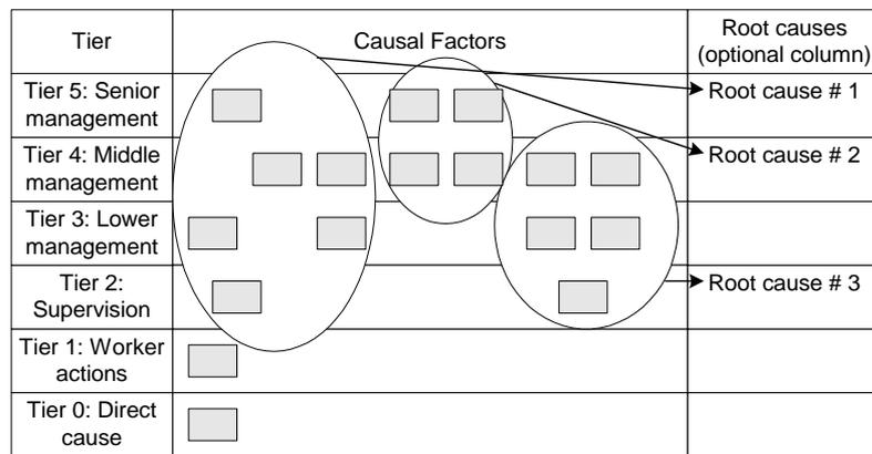
Figure 13. Identifying the linkages to the root causes from a TIER-diagram.
