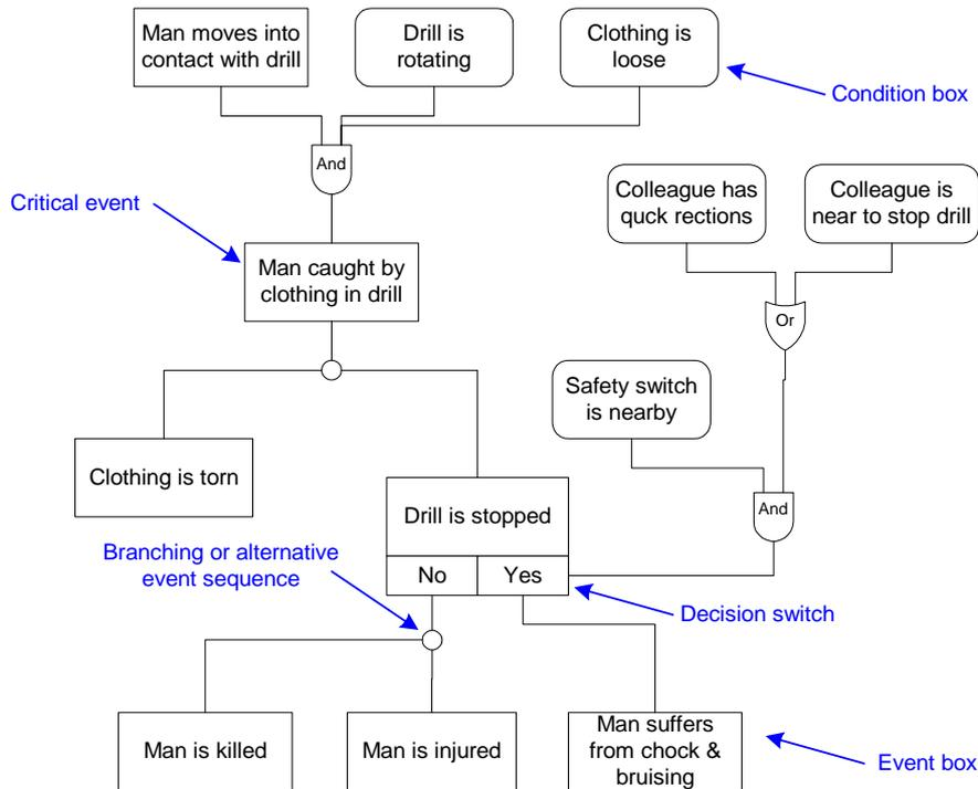
Figure 33. Cause-consequence diagram.
