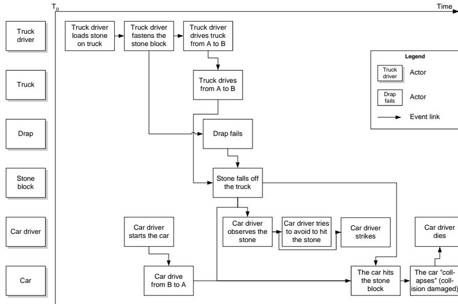
**Figure 23.** An example on a simple STEP-diagram for a car accident.
