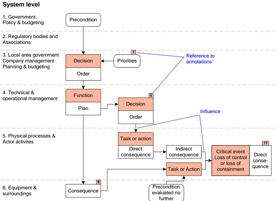
**Figure 34.** An approach to structure an AcciMap and a proposed legend of symbols.
