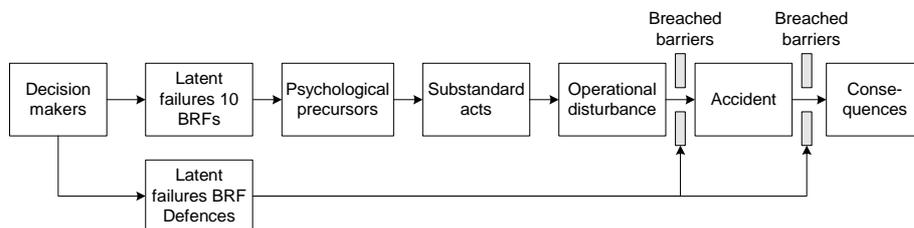
**Figure 28.** The complete TRIPOD model.
