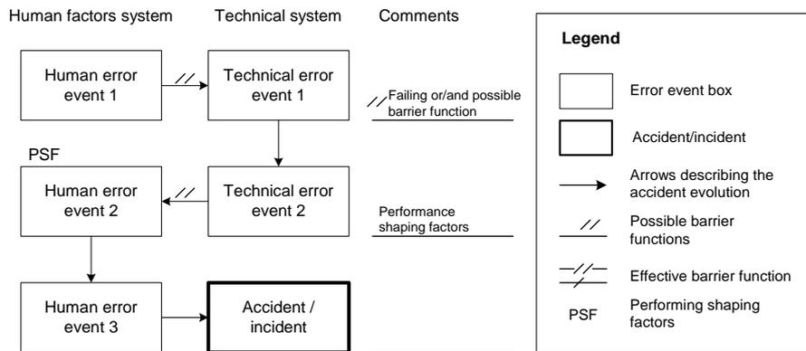
**Figure 27.** Illustration of an AEB analysis.
