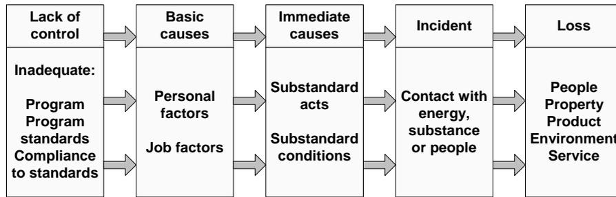
**Figure 18.** The ILCI Loss Causation Model (Bird and Germain, 1985).
