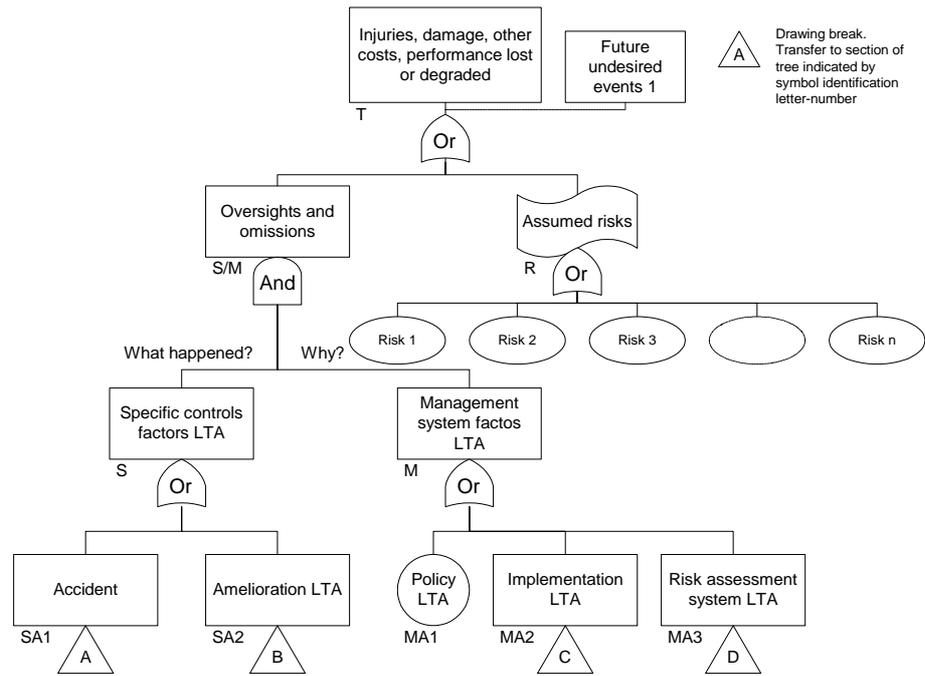
**Figure 17.** The upper levels of the MORT-tree.
